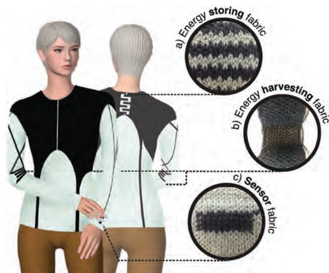
Figure 1. Seamlessly knitted MXene-coated cellulose-based yarns. Concept illustration of a garment integrated with energy storage and harvesting device with a capacitive pressure sensor. Insets show actual device prototypes comprising of a) knitted energy storing fabric with alternating MXene-coated cotton yarn (black) and a nonconductive commercial viscose yarn (green). b) Knitted energy harvesting fabric with alternating MXene-coated linen yarn (black) and a commercial Teflon yarn (brown) can be placed strategically to harvest energy from body movements. c) Capacitive pressure sensor device knitted with MXene-coated bamboo yarn, where the device can sense different applied pressures ranging from low to high.
